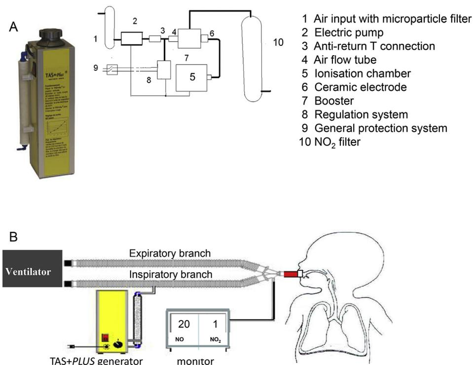
**Fig. 1.** Schematic representation of the TAS + PLUS device generating NO from the air and its connections. A. A picture showing the device and a diagram representing the different parts are shown. B. The device is connected to the inspiratory branch of the mechanical ventilator and the concentration of NO delivered to the neonate is measured with a monitor connected to the Y-piece of the endotracheal tube of the newborn.
